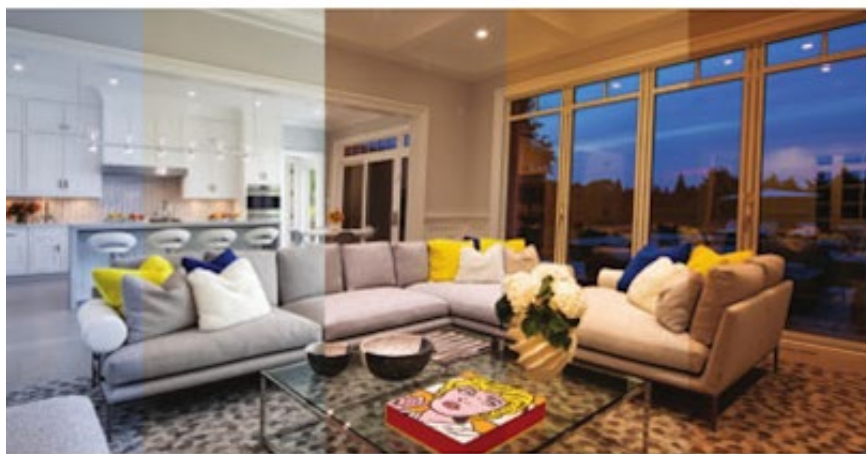
The living space showing the changing color temperatures from left: 5000K, 4000K, 3000K, 2700K and 2200K.
