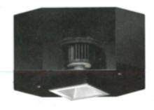
MKS Advanced LED 5" Downlight Series, Sunlite Manufacturing • This series of insulation-contact-rated, baffle-trim LED downlights is offered in round and square 5" apertures. The white baffled trim houses a recessed, convex diffusing lens made of impact-resistant polycarbonate. Consuming only 20W and delivering between 1,000 lumens and 1,780 lumens, the Nichia LED source is available in 3000K, 3500K, and 5000K with a CRI of 80. • sunlite.com • Circle 296
