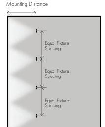
Wall Wash Mounting Recommendation: Mounting Distance = 2'-0" - 3'-6"Fixture Spacing = 2'-6" - 4'-0"
