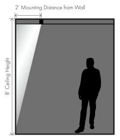
Need help determining the perfect wall wash layout? Contact USAI for applications assistance.
