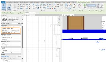
\*Workplane-Based files show elevation from level field in properties window, which gives the ability to edit mounting height
